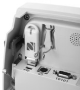
Interface connections inside of the Terminal.
